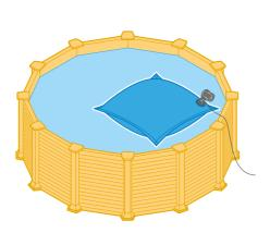
Inflate the pillow to about 60% to 70% (two-thirds) of its full capacity through its hermetic dual Boston valve that's compatible with any blower.
