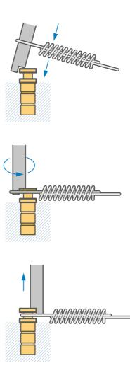
7 When the anchors are installed, use the rod to pull the springs and make them slide over the anchors.
