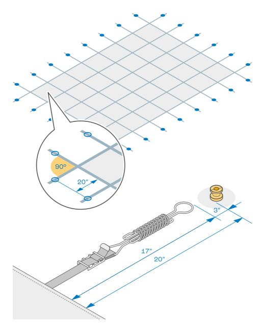
Using chalk, mark spots on the deck where holes need to be drilled for the anchors. Start with the central straps (first lengthwise, then widthwise): the distance between the holes and the edge of the cover should be approximately 20". Once you mark spots for central holes on all four sides, move outwards towards the corners of the cover. Drawing chalk lines between the spots will help make sure that all the holes will be drilled at equal distances from the edges of the cover.
