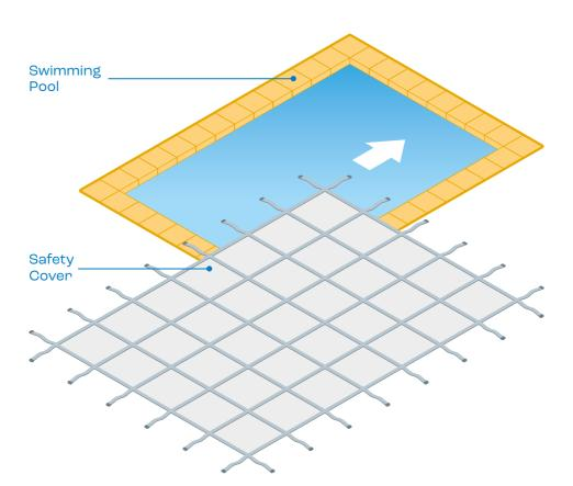
Unfold the cover carefully and spread it out on the water in the pool. Make sure there's enough water in the pool to support the cover during installation.
