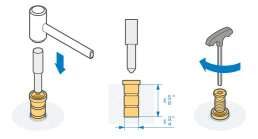
5 Drill the holes and install the anchors.
