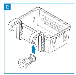
Attach the regulator between the hooks.
