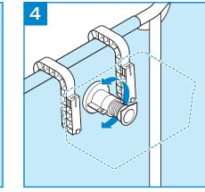
Twist the regulator to make it longer or shorter until the basket's bottom is at the right angle to the pool wall.
